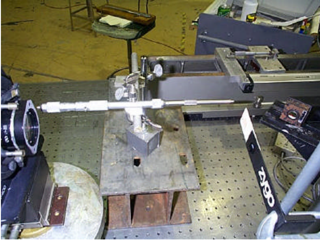
Figure D3 Inside micrometer prior to alignment
