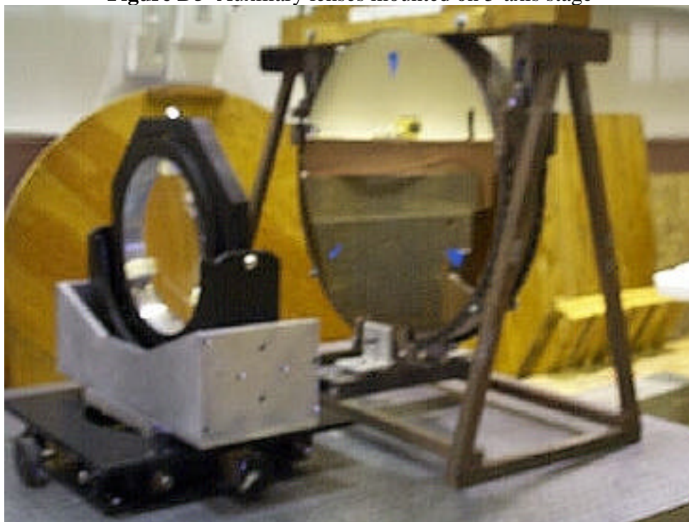
Figure D6 Lens 3 in 5-axis mount and return flat
