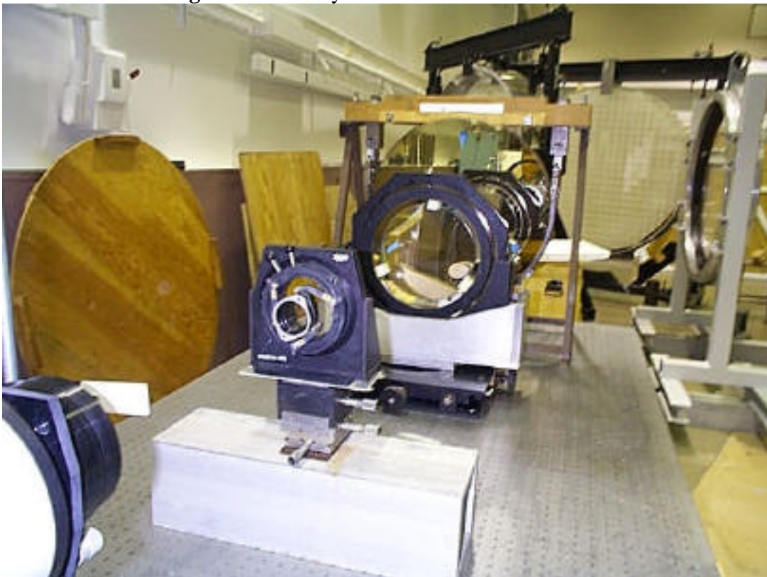
Figure D8 Test system as seen from interferometer
