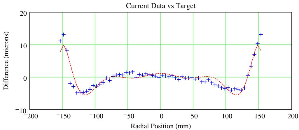
This plot compares the current asphere fit to the data with the target asphere:
