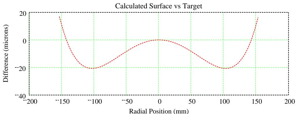
This plot is the difference of the new data and the old data, a measure of removal:
