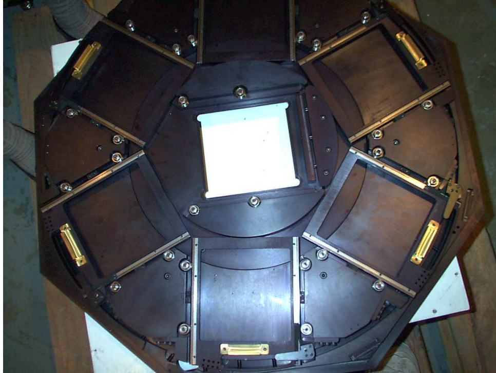
Figure 6. The 90prime filter wheel.
